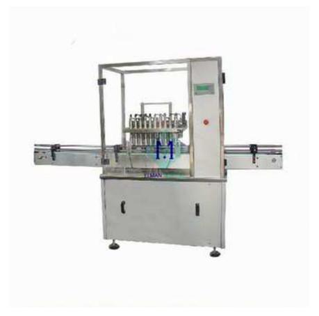
The Bottle Air Rinser is used to automatically remove dust, dirt and other foreign matter. Its dual action nozzles first blows high pressure air into the container to dislodge dust and debris and then vacuums the dust and debris from the inside of the container. It frees dust and dirt through ionized air to neutralize any static electricity that may be on the containers, guaranteeing an elevated cleaning process.
