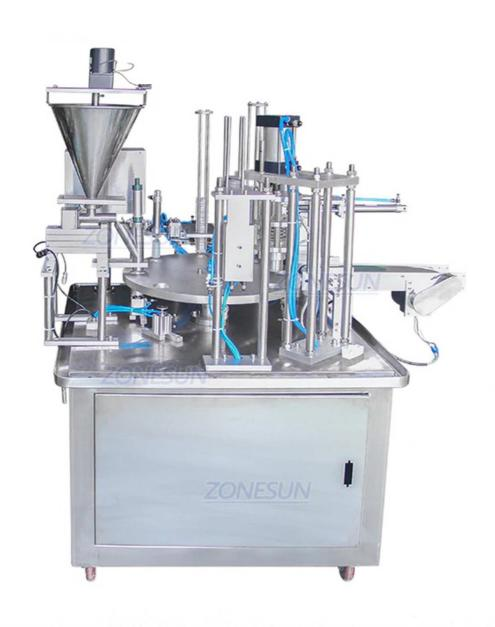
This rotary coffee capsule-filling machine can feed cup, fill powder, seal cup cover automatically at the same time. The filling speed and sealing temperature can be controlled easily, and we can customized this machine to make it suitable for your products according to the diameter of the container.
