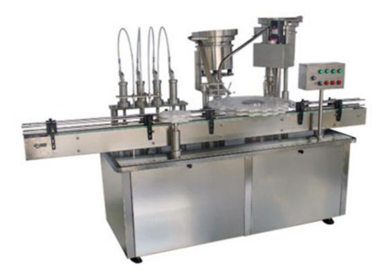
This type of equipment is the update version form TTG-I filling and capping machine according to the requirement of market. It applies widely to pharmaceutical, food and chemistry industry. It integrates the function of filling, stoppering, capping into one machine, and feature of compace structure, volume economy, both of round bottle and abnormal bottle are suitable for this machine.
