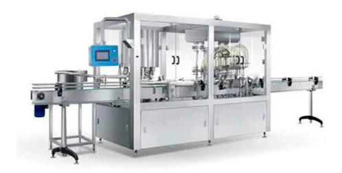
Syrup Washing Filling Capping Machine includes syrup bottle air /ultrasonic washing, dry syrup filling or liquid syrup filling and capping machine. It is integrate design, one machine can wash, fill and screw bottle in one machine, reduce investment and production cost. The whole machine is with very compact structure, small occupying area, and less operator. We can equip with bottle handing and labeling machine also for the complete line.
