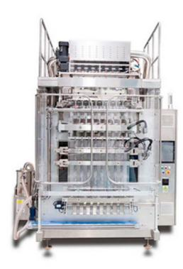
Stick pack is mainly for packing the powder into the sachet, plastic bag. It is mainly suitable for sugar, milk powder, starch, the coffee, condiment, soild drink packing. it can measure, fill, bag making and Date print. It is one automatically Sachet packing machine.
