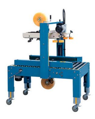
The CHS-6603A carton sealer is an automatically adjustable auto carton sealer. It enables every operator to start production easily because it is easy to use and adjust different cases. With top & side driving belts for the transportation of cartons it performs the sealing of the box. According to customer requirements 2' or 3' tapping heads can be included. Carton sealers have been designed and manufactured according to CE Standards.
