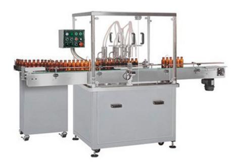
Automatic Six/Eight Head Volumetric Linear Liquid Bottle Filler Machine (Model SBLF-200) is suitable for bottles with max. Speed of 160 bottles/minute. Unique twin track operation of bottles gives easy bottle movement at lower speed and generating high output.
