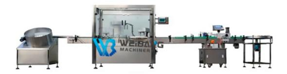
Application: the machine is mainly used for filling and capping syrup, honey, fruit juice, wine, beverage, soy sauce, vinegar, cod liver oil, olive oil, essential oil, hair oil, ink, disinfectant, injection, washing liquid and various medical liquids.
