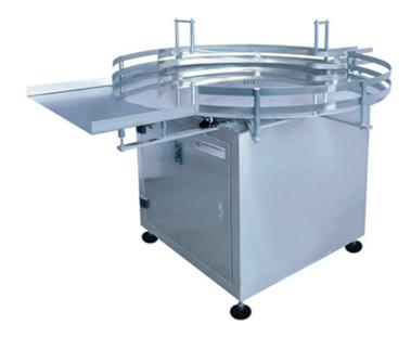
The automatic transmission is suitable for round bottle, square bottle, such as conveyor belt connected to the labeling machine, filling machine, capping machine, automatic bottle feeding, improve efficiency; can be applied to the intermediate junction line, as a buffer platform, shorten the length of conveyor belt. Applicable bottle range can be adjusted freely, bottle conveying speed 30~200 bottle / minute, speed can be stepless adjustment, convenient production arrangement.
