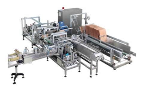
LWP-3 Series Auto-packing Machine is a patent product of Guangzhou Leiwest Pak Co., Ltd. Depends on the effective and stable process from auto-ranking of packs to auto-molding and sealing of boxes, the packing machines can work automatically. A revolutionary function, automatically insert cystosepiments has been achieved.
