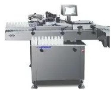
Suitable for all kinds of square, round, oval and various irregular curve bottle sleeves. It adopts the box buffer type labeling mechanism and has good buffering performance. Using imported famous brand servomotor, the labeling speed is fast, the precision is high and the stability is good. The single-slide belt drive is used for both the pull-tab mechanism and the cutter holder. The transmission precision is high and the replacement is convenient.
