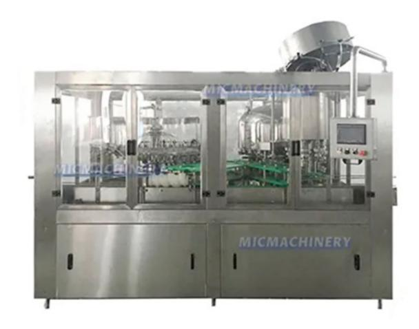
MIC 24-24-8 Small Beer Bottling Line is applicable for glass bottle filling capping machine for craft Beer
