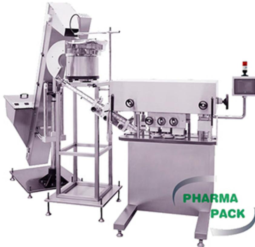
The capper LFCL-15F is a reliable, high performance machine, designed in conformance with current and proposed GMPs. Having a small footprint, they are effective in maintaining the integrity of a clean room environment. Few change parts needed for different cap sizes (only the cap slide rail). The machine is designed for maximum efficiency and versatility. It utilizes the latest technology to automatically place and precisely torque a wide spectrum of cap types onto virtually any bottles type.
