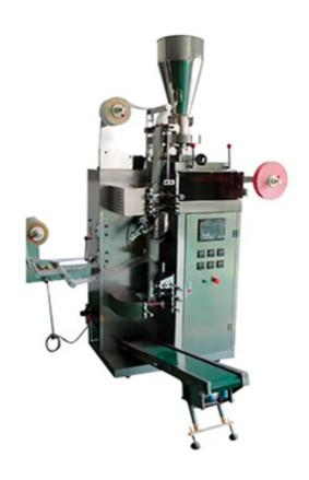
This machine is suitable for automatic packaging of seed, medicament, health products and tea etc industries, such as seed, healthy tea, traditional Chinese medicine and tea bags etc. Principle of work: First the raw materials are filled into the inside bag, then put the inside Bag in the outside bag by magic hand.
