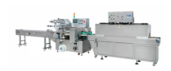
There are 2 model of Horizontal Flow Wrappers. One is PSA-250NS for non-shrinkable film, another one is PSA-250WS for shrink film; it must work with heat tunnel.
