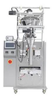
DXD-300F Automatic Powder Packaging Machine is suited for the continuous filling of many different types of powders with fluidity and loose packing density, such as flour, coffee powder, lotus root powder, soy milk powder, milk powder, bone strengthening powder, granules, nutraceuticals, and other materials.
