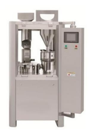
NJP-200C/400C/800C automatic capsule filling machine is suitable for filling various capsules. It can automatically complete positioning, separating, filling, waster capsule rejecting, locking and finished capsule ejecting. This automatic capsule filler is the ideal equipment for filling capsules especially in medium and small pharmaceutical factory, hospital preparation lab, and so on.
