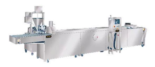
The RPS Series is designed with water spraying, steaming, softening, and filling devices, so workers only need to put rice papers on the conveyor and fold the spring rolls. You can also add a lifting device to place rice papers automatically.
