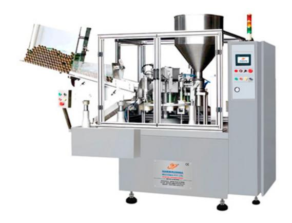
The Automatic Tube Filling, Sealing and Coding Machine consist of a main structure, tube moving with a tube holding unit, safety acrylic enclosure (OPTIONAL), jacketed hopper with a stirrer (OPTIONAL), filling nozzles, sealing head, coding unit, hot air sealing unit, electrical panel, PLC & HMI (OPTIONAL), mains on/off & motor.
