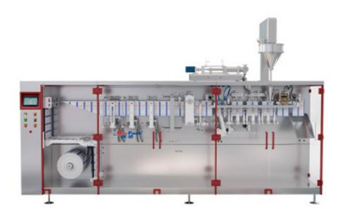
Horizontal twin pack sachet packing machine is an ideal bag packing equipment that meets the requirements of high-quality packaging and smaller bag type. The packaging speed is fast and can realize the three-side sealing and four-side sealing bag types. This machine is suitable for powder, particle, liquid, paste, solid, and other materials packaging needs; Roll film molding reduces the cost of packaging.
