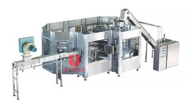
The machine is mainly used for filling carbonated drink. It combines rinsing and filling and capping as one automatic body suitable for PET or other plastic bottles. The iso-pressure (iso-barometric) filling technology is adopted enabling it to fill more efficiently and more stably with more output than the machine of the same level from others.
