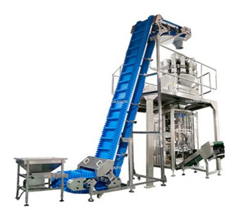
This unit machine is special design for packaging frozen food like shrimp, meat ball, Chicken pieces dumpling and Toufu in to plastic bag. The whole machine have the function of automatic product feeding, weighing, film bag forming, bag sealing ,Including date coding, bag counting. The finished bag is output from conveyor machine which no need manual collect the bag and avoid the bag polluting.
