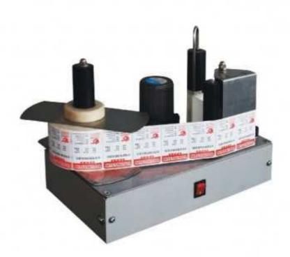
Labeling machines are applied to various operations such as sticking a label on plane, post surface, single side or multi-sides of a package, sticking labels covering part or all of the surface of a cylinder, or sticking on sunken locations and at edges or corners.
