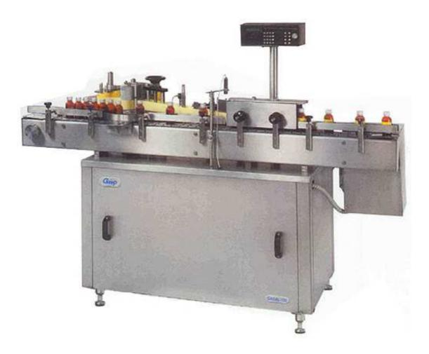
The Automatic Vertical Sticker Labeling Machine GASAL-150 is one of the most users friendly. The machine is used for full/partial wrap around labeling on different size of round container. It is capable of labeling up to 150 containers per minutes depending on products and label size. The automatic model is equipped with roller spacing device resulting in a simple to "No change parts required".
