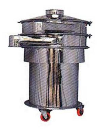
Crevice free GMP design; Super tight finish; Bio safe Toxicology Tested; Calibrated & Certified as per International Standards.; Available in S.S 316 and S.S. 304 Quality; Available in sizes ranging from 30 mm dia to 1220 mm dia.; Import Substitute Designs; Wire Mesh sizes available from 2# to 600 # as per all International Standards.;
