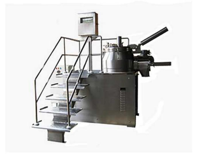
Rapid Granulator Mixers designed to meet special needs of tablet manufacturing technology. This is achieved by reducing processing time, more homogenous mixing, Uniformity of Granule size and above all maintaining improved hygiene compliant to GMP norm.
