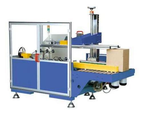
The CHS-6701 is a Vertical type Automatic Carton Erector. This system fits for automatic production line. It erects cases of different and sizes and it seals the bottom side of carton with tape or hot glue on demand.
