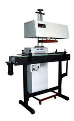
Continuous induction sealing machine utilizes electromagnetic induction principle to produce instant high heat to melt aluminum foil that then adheres to the bunghole, reaching the aim of wet-proof, leakage-proof, mildew-proof and extending preservation time. Now it is widely used as sealing package machine in industries such as pharmaceuticals, pesticides, pesticides, lubricant and cosmetics etc.
