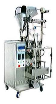
The MK-214 is a fully pneumatic vertical form fill and seal (VFFS) packaging machine designed to package various powder products. This Fully automatic vertical packaging machine uses auger screw dozer filler system to produce center sealed, 3 side sealed and 4 side sealed pouches / bags.
