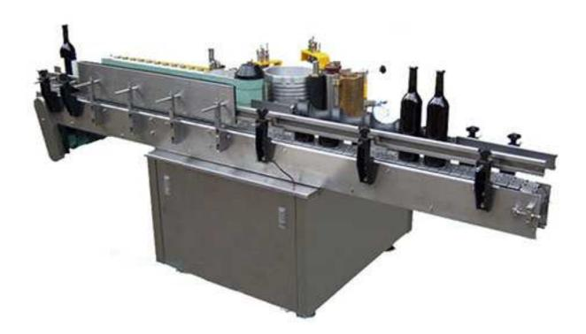
It is a double side's glue label machine, both front &back labels charged by the two labeling applicators respectively, delivering labels, delivering bottles, pasting and labeling are finished at a time automatically, and the front & back labels will also be pasted on the bottle in the same time. Adopt touch screen operating, PLC controlling, pneumatic pressing bottle labeling
