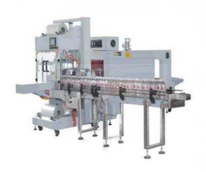
QSJ-5040A is suitable for wrapping products such as pop-cans, bottles, etc, with bottom-tray or without bottom-tray, working with BSE-6040 or other PE shrink tunnels.
