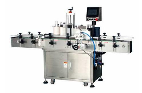
OLR-R is economical, self contained, easy to operate, equipped with auto teach programming touch screen. Built in microchip storing different job setting makes fast and easy changeover. This automatic labeling system can orient label precisely for cylindrical container.
