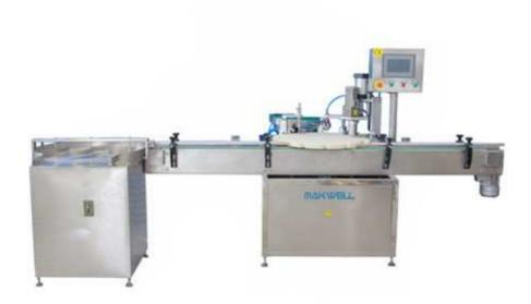
Automatic pharmacy liquid filling machine is a high-tech product researched and developed by our company. It is suitable for products of liquid such as oral liquid, liquid chemical etc. It is widely applied for filling of products in such industries as food, cosmetics, medicine, grease, daily chemical industry, detergent, pesticide and chemical industry etc.
