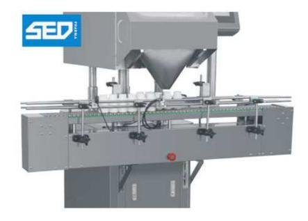
SED-8SII Electronic Pill Counter Pill Counting Machine is suitable for pharmaceutical, food, and chemical industries. It automatically fills bottles with pills or tablets, then counts and covers the bottle. It can be connected with next process. Being beautifully designed and easily regulated. It is an ideal choice for packing for packing and counting equipment.
