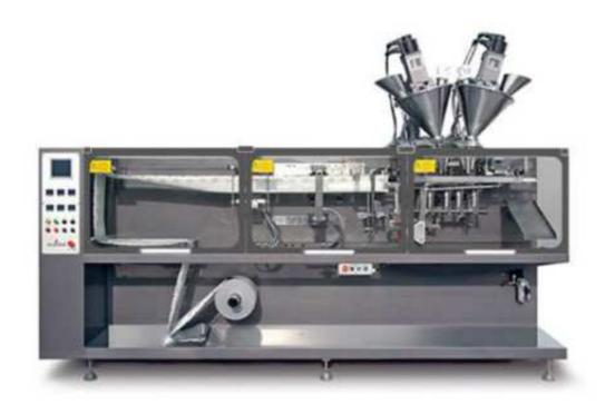
The machine can be used for various heat sealing multilayer compound membrane materials packaging. Automatically finish forming, such as bag making, filling, and sealing packaging process. Choose different filling device can be suitable for different packing products. For example: power, paste, granule, liquid and so on.
