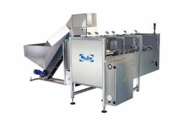
Randomly oriented bottles are received in bulk into the hopper and supplied to the centrifugal disc by means of a conveyor. In the disc, the bottles are guided into a qualified position suitable for the stand up unit to process them into the required discharge position Symmetrical bottles are stabilized and released on the customer conveyor.
