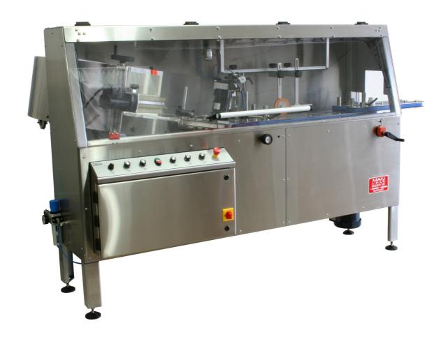
Acasi manufacturers bottle unscramblers that are used to automatically feed empty containers into the production line. The bottle unscramblers we manufacture are limited to plastic, metal and non-fragile containers.
