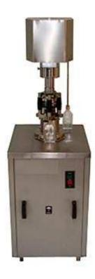
Suitable for ROPP Capping, Screw Capping, CRPP Capping, Crown Capping, Dosing Cup Sealing
