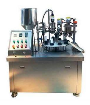
This semi auto tube filling and sealing machine is widely used in pharmaceutical, cosmetic, food and chemical industries etc. It is applicable in various aluminum plastic compound soft tube, plastic soft tube which fill pack all kind of Such as ointment, adhesives, AB glue, Neoprene, epoxy glue, skin cream, hair cream, boots oil, toothpaste and else liquid, lotions and cream etc.
