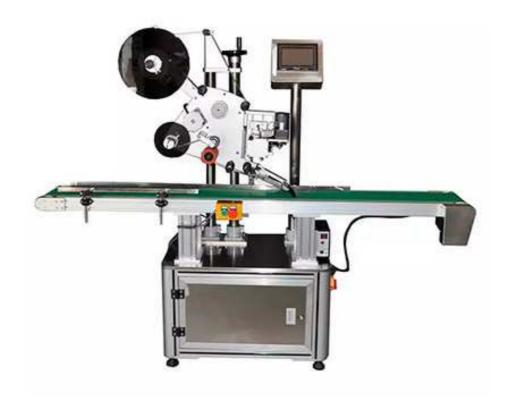
This Automatic Flat Labeling Machine is applied to label the self-adhesive label on various flat surface products, as books, file folders, cases, cartons, bags, etc. This machine is widely used in electrical, pharmacy, foodstuff, beverage, cosmetic and chemical etc industries.
