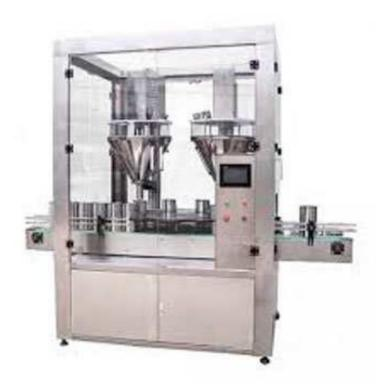
Dual heads automatic auger filler is a high-end auger filler developed by Vtops Machinery. This machine equipped with two auger-fillers for different functions: high-speed filling, or high-precision filling, or filling-by-vibration, or filling-by-weighing. It is ideal for high-end customers with special needs.
