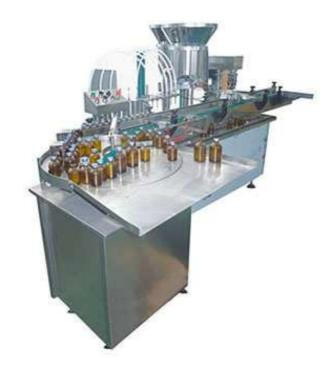
This vial filler and capper is specially designed for filling, capping and sealing 1-50ml penicillin vials.
