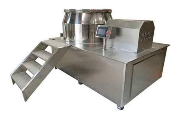
The powder raw material and adhesive in a cylinder ate mixed fully at the bottom to become a humid soft material. Then it is cut through high-speed crusher and become uniform granules.
