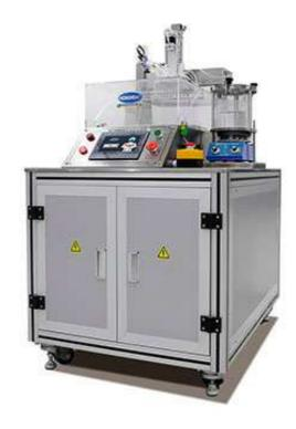
Test Tube Filling Machine is used for clot activator BCA dosing spraying for blood collection tube. It uses imported pinch valve with 10 nozzles for effective, even spraying, and there is automatic cleaning device for the nozzles, easy and time-saving for maintaining. This machine is equipped with magnetic stirrer and refined atomizing nozzles, which can provide you more stable and quality working performance.
