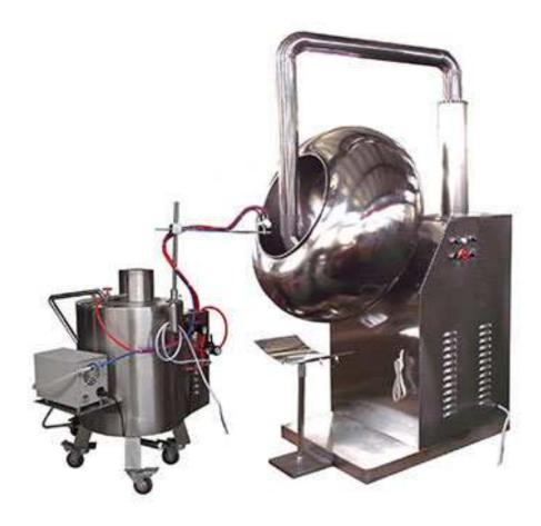
This machine is used to carry out sugarcoating and film coating to the core of Chinese traditional and Western medicine tablets. It integrates strong power, weak power, hydraulic and pneumatic. It is new type equipment improved on the basic of original common type sugarcoating machine.
