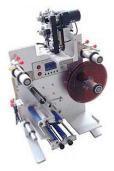
This machine label 1 round bottle with 2 labels, so long as the 2 label's length is same. This label machine is used for labeling and coding on various round bottles, coding, such as: glass bottles, plastic bottles, cans and so.
