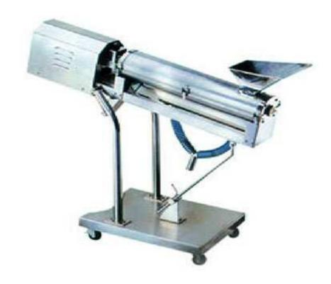
KW-108 polishing machine is used after capsules ware for cleaning the powder attached on the capsule surface, through mechanically orating brush and attraction of vacuum to take out the externa.
