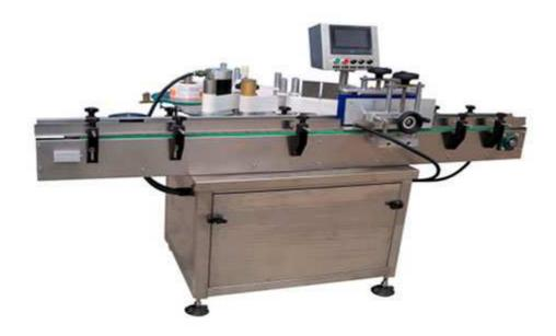
With automatic detection of bottles and labeling size, labeling accuracy, automatic parameter adjustment, two options of "stepping traction" and "servo traction" for the speed control.
