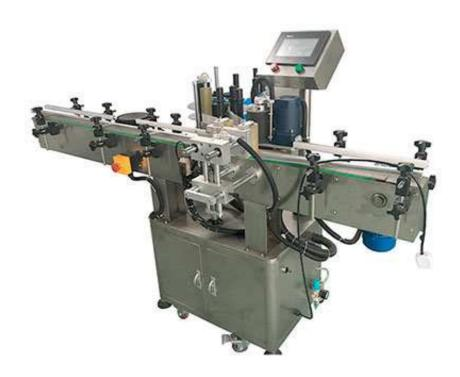
Adhesive Stick labeling machine for Top is special for stick the label on the top of cap
