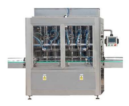
The filling system is driven by servo motor which assure high filling accuracy, also easy to set filling volume on the touch screen directly.
